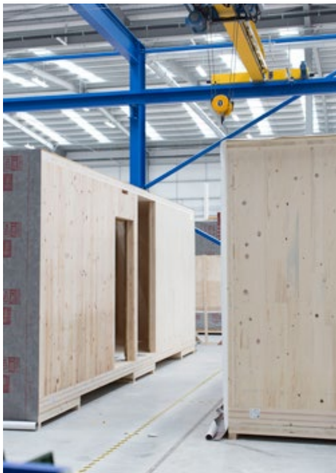
CLT modular units in a factory environment
